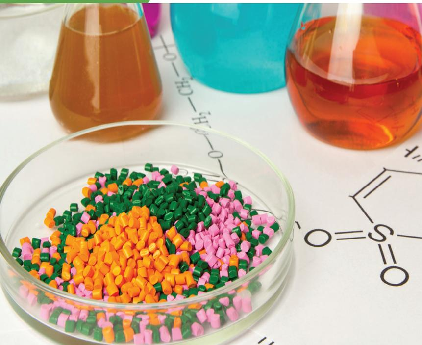
ABS is comprised of three components, acrylonitrile makes it robust, butadiene provides a rubber-like toughness, and styrene, provides a high-quality glossy surface. Making it tough, durable and visually appealing all at the same time.
